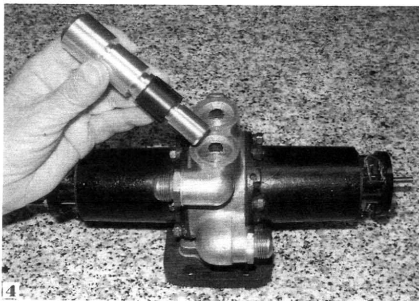
4 Valve seat lapping tool generated from a left over project from lathe school.
