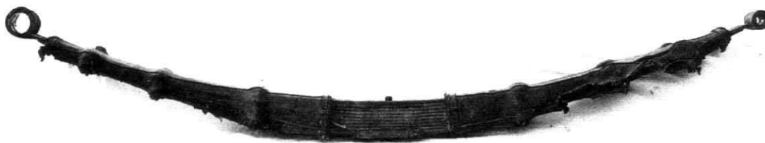
Figure 1: Rear semi-elliptic spring from Phantom III, 3BU86, still gaitered, and prior to disassembly.
