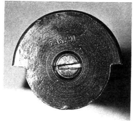
Figure 3: Typical shackle pin that has not been receiving adequate lubrication. Note the worn areas where the bushings were, and the slightly damaged thread where the pin was driven out (with the nut on, please!). The center oil hole was so blocked that it had to be drilled out. Figure 4: End of shackle pin after cleaning and removing the solder that sealed the screw. A well-fitting screwdriver and heat, used together, are needed to remove it.
