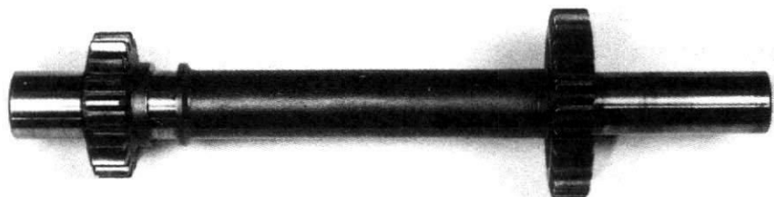
Reverse motion shaft. This rides in a white metal bearing, which is quite delicate. High-speed reversing is not recommended in your Small Horsepower Rolls-Royce or Derby Bentley.
