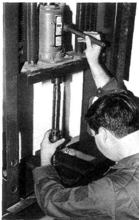
Pressing the roller bearing onto the rear of the second motion shaft. The author's left hand is on the second speed sliding gear.
