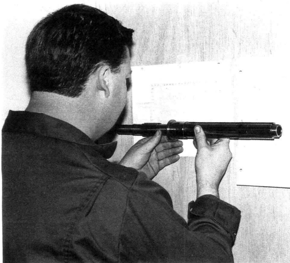
Using the Schematics and General Arrangements Drawings is a must. Here the author compares the second motion shaft to the drawing from the Service Sheets.
