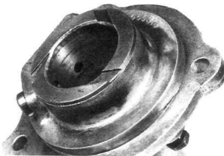
White metal bushing for reverse motion shaft. If out-of-round or worn through at any points, it will have to be re-metaled and rebored by a specialist.
