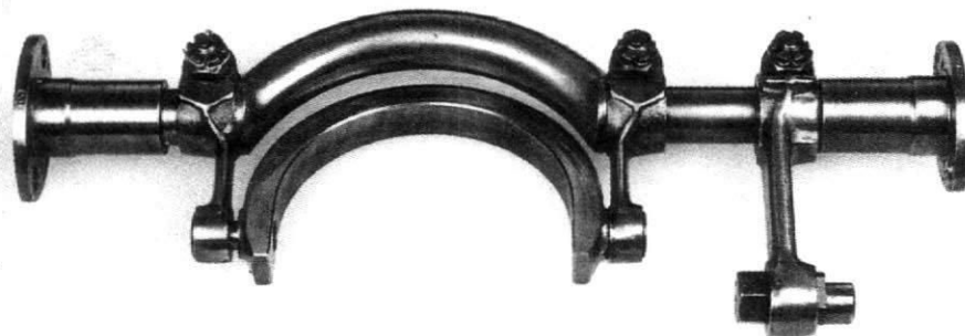
Synchromesh actuator and bushings. Do not disassemble this unit further, as it is fitted and aligned at the factory. Clean the unit as a whole.
