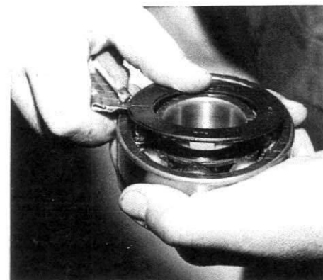
Removing the seal from a bearing. Use a sharp knife to simply pop the seal off.
