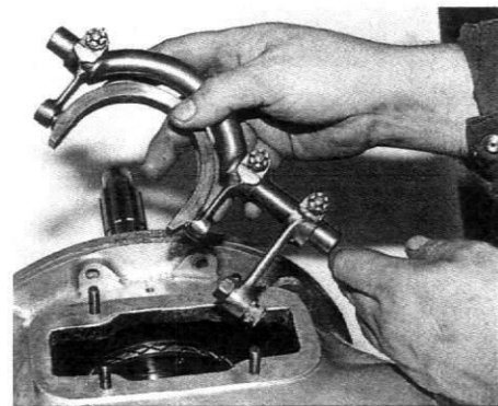
Inserting the synchronesh actuator unit. It goes in only one way, so if it does not drop into place instantly, lift out and try again.
