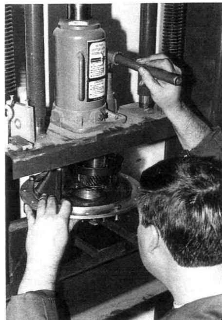
Pressing the first motion shaft into the bearing in the diaphragm. Support this aluminum casting well. You don't want to break or warp it.
