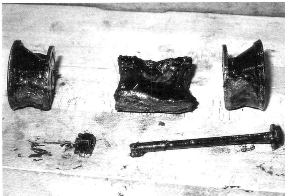
7 The crankshaft has hollow journals that fill with oily sludge as a result of the centrifugal-like action of the spinning crankshaft. Aluminum plugs seal the ends of the journals and are held in place by through-bolts. The plugs should be removed and the sludge cleaned out so that oil flows freely to the big ends of the connecting rods. Note build-up of sludge in journal.
