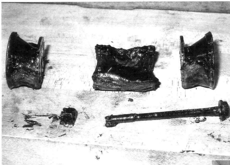
8 Aluminum sludge trap seals showing build-up of oil sludge and plug of sludge (middle) removed from journal.
