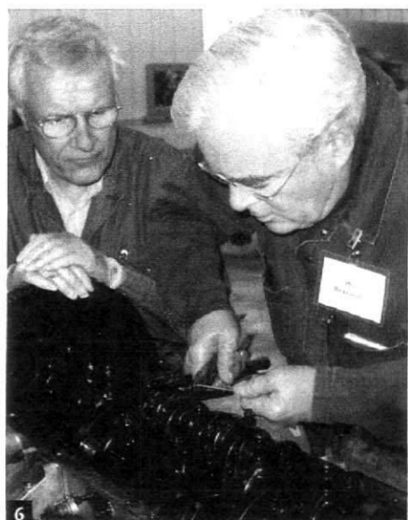
6 Peter Sedmihradsky (ONT) and Phil Birkeland (WA) work on removing the numerous cotter pins securing the castellated nuts on bearing caps.
