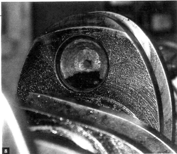
70% occluded crankshaft journal (courtesy Dennison-Jayne Motors).
