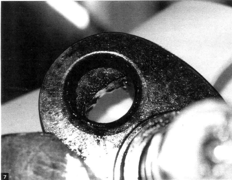
7 The crankshaft has hollow journals that fill with oily sludge as a result of the centrifugal-like action of the spinning crankshaft. Aluminum plugs seal the ends of the journals and are held in place by through-bolts. The plugs should be removed and the sludge cleaned out so that oil flows freely to the big ends of the connecting rods. Note build-up of sludge in journal.
