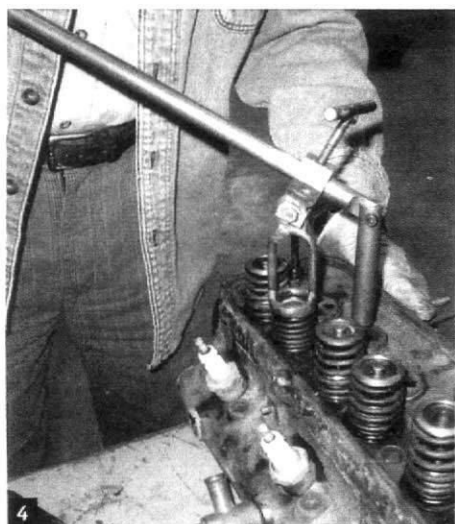
4 Shop-made tool to compress valve springs. The end is threaded \frac{1}{16} " BSF and screws on to the rocker arm bolts. The handle has a sliding arm to center the tool over each valve spring. This design allows you to remove the two valve springs closest to each rocker arm bolt.
