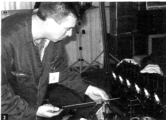
2 Tim Jayne uses a long screwdriver with tip ground to exactly fit the 2BA screws that hold on the side plates on the block.
