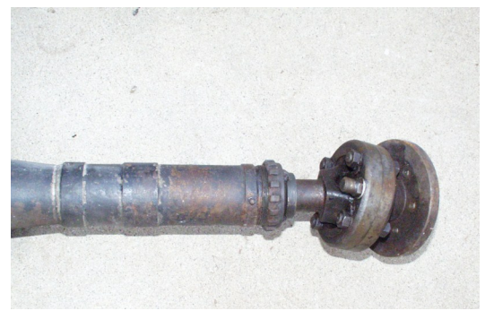
U-7 Drive Shaft-No Damper
