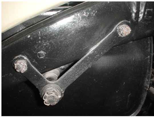
U-6 Fuel Tank Hanger
